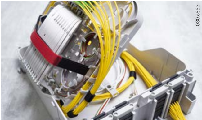
Swivelling fiber inlay for safe separation of incoming and outgoing fibers
